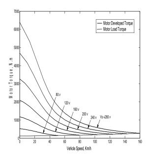
Figure 6. The motor torque versus vehicle speed during acceleration.
