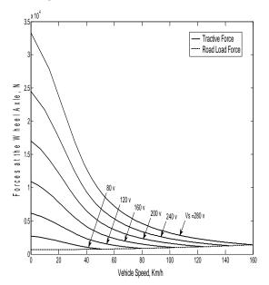
Figure 4. Tractive and resisting forces at wheel axle versus vehicle speed during acceleration.
