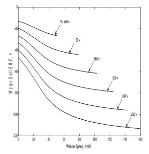
Figure 13. Motor self EMF versus vehicle speed during acceleration.
